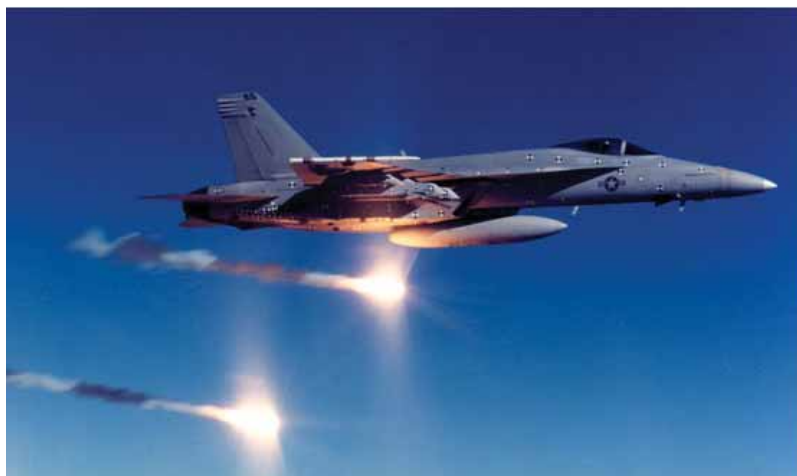
Figure 36. Navy F/A-18E Aircraft Dispensing IRCM Flares.
